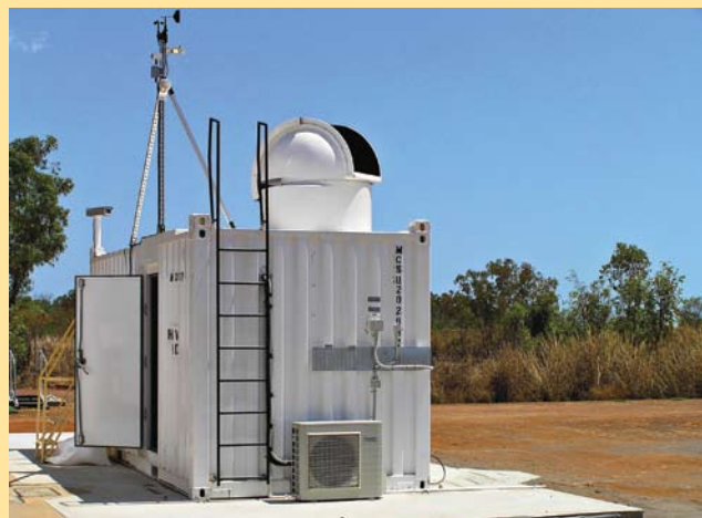
The TCCON observatory in Darwin, Australia. The Total Carbon Column Observing Network (TCCON) is a ground-based network of high resolution Fourier transform spectrometers (FTSs) which retrieve high-quality column-average mixing ratios of CO 2 , CH 4 , N 2 O and several other gases. Total column measurements of CO 2 are tied to the WMO calibration scale through comparisons of FTS data with integrated aircraft profiles measured over TCCON stations with in situ instruments themselves calibrated to the WMO scale. TCCON data are insensitive to vertical transport processes and can be used for verification of forward and inverse models. Furthermore, they serve to validate total column CO 2 and CH 4 satellite measurements from for example GOSAT and SCIAMACHY. TCCON was established in 2004 and joined GAW as a contributing network in 2009. Many of the current measurement sites are also part of the GAW-affiliated Network for Detection of Atmospheric Composition Change (NDACC). TCCON currently has 13 observation stations from Spitsbergen in the high Arctic to Lauder, New Zealand. For further information see the TCCON web site ( http://www.tcon.caltech.edu ). Photo: David Griffith, University of Wollongong, Australia.
