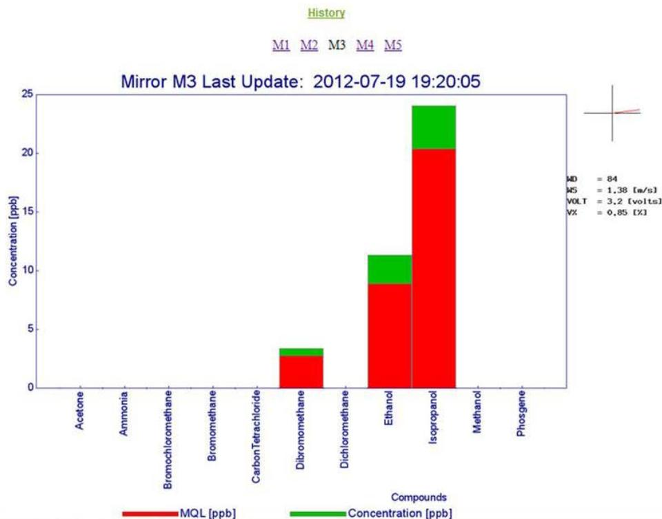
Incorporating synchronized wind data may direct site personnel to the area of major leaks. Real-time data access is via a password-protected internet site.
